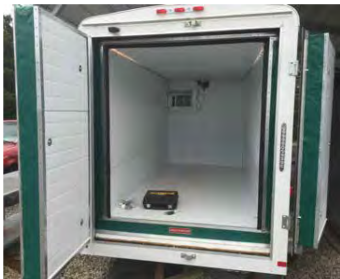
Figure 13. The cooler complete with trim and weather-stripping.
