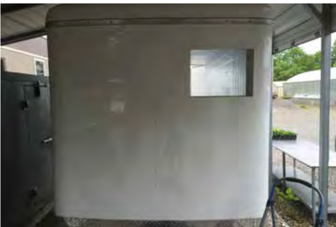
Figure 9. Cut a hole in the front of the trailer for the AC unit with a counter rotating circular saw.
