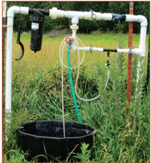
Figure 2. A venturi-type injector introduces fertilizer into the irrigation water.
