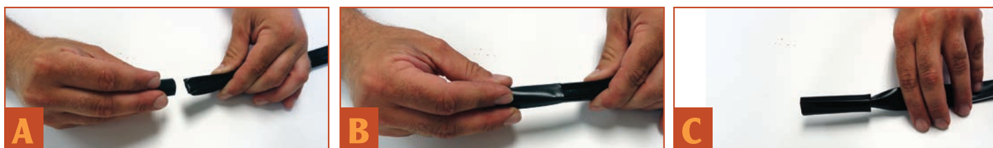
Figure 12. (A) Fold the drip tape three times and hold securely. Crease and bend the folded end lengthwise to make it easier to place the sleeve over the end. (B) Slide the sleeve (~2-inch piece of drip tape) over the end until it is completely covered (C) to keep it from unfolding when pressurized.
